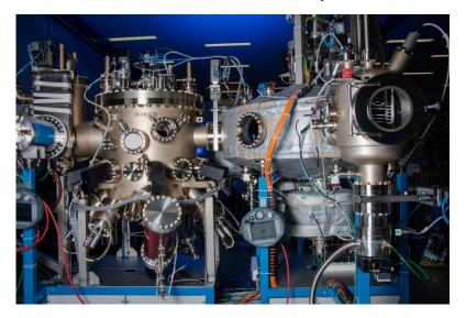
A new Asian customer has just ordered an automated MBE 412 machine to strengthen its fundamental and advanced nitride research capabilities. This MBE 412 machine will be used to develop optoelectronic devices for end-use applications such as light-emitting diodes, UV sensors and microwave power components.
